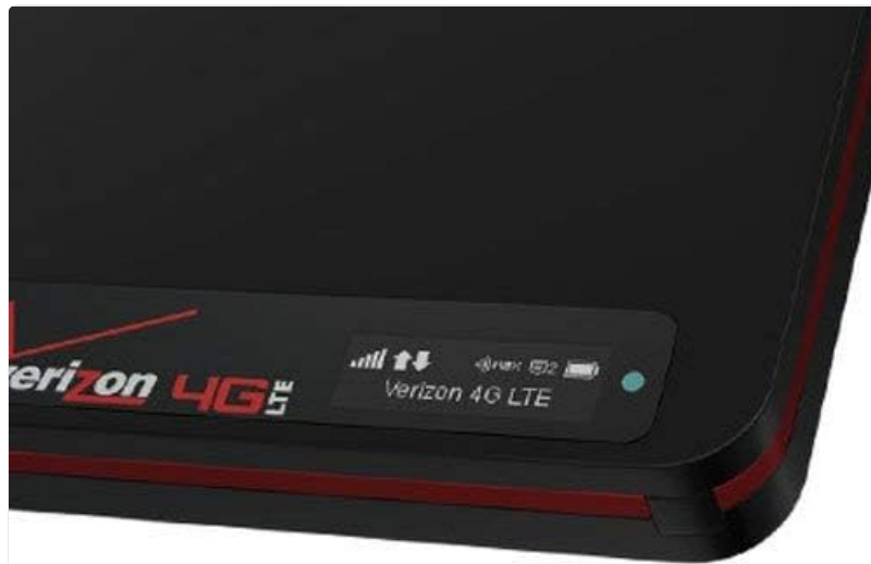
Image: Close-up view of the Jetpack's OLED display, showing signal strength, battery level, and network type (Verizon 4G LTE).
