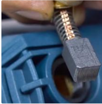
Image 6.1: A carbon brush, a replaceable component in the saw's motor. Regular inspection and replacement of carbon brushes are crucial for maintaining motor efficiency.
