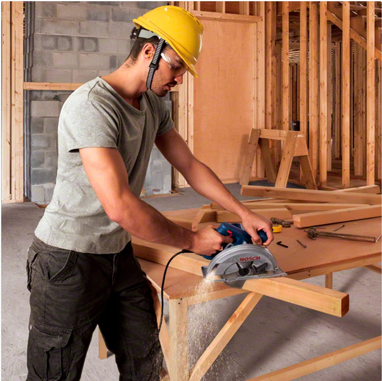
Image 5.1: A user demonstrating a straight cut with the Bosch GKS 150 Circular Saw. The user is wearing appropriate safety gear and maintaining a stable posture.
