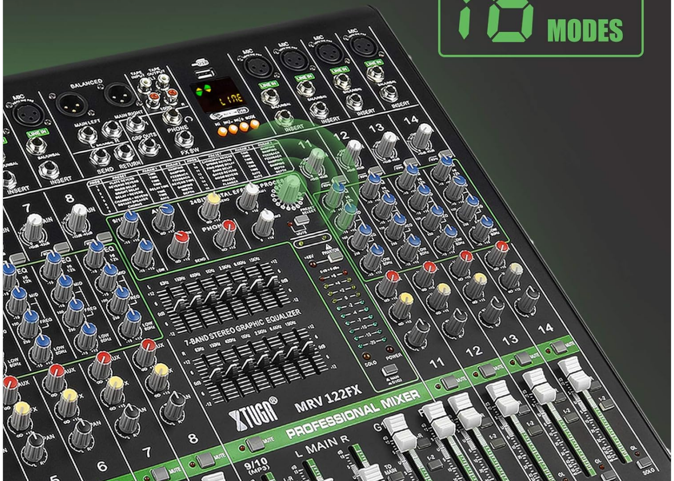
Image 4.3: Section of the mixer highlighting the 24-bit digital effects processor with 16 modes.
