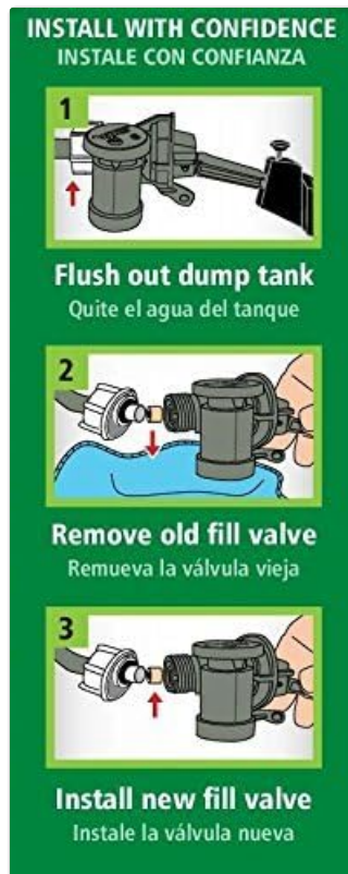
Image: A visual three-step guide illustrating the installation process: 1. Flush out dump tank, 2. Remove old fill valve, 3. Install new fill valve.
