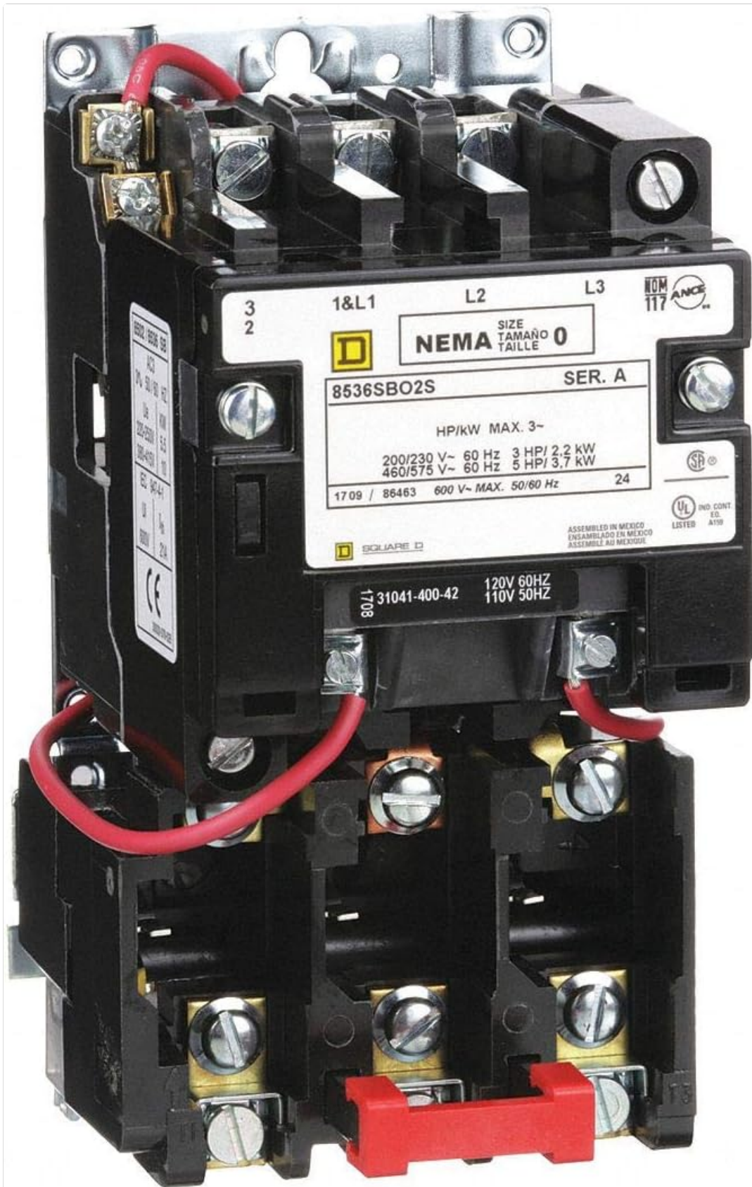
Figure 1: Square D Magnetic Motor Starter (Model 8536SBO2S). This image displays the front view of the motor starter, highlighting its NEMA Size 0 rating, model number 8536SBO2S, and coil voltage of 120V 60Hz / 110V 50Hz. Visible are the main power terminals (L1, L2, L3 at the top, and T1, T2, T3 at the bottom), the control circuit wiring (red wires connected to the coil), and the maximum horsepower/kilowatt ratings for 3-phase operation (e.g., 3 HP / 2.2 KW at 200/230V, 5 HP / 3.7 KW at 460/575V). A red reset button is located at the bottom of the unit.
