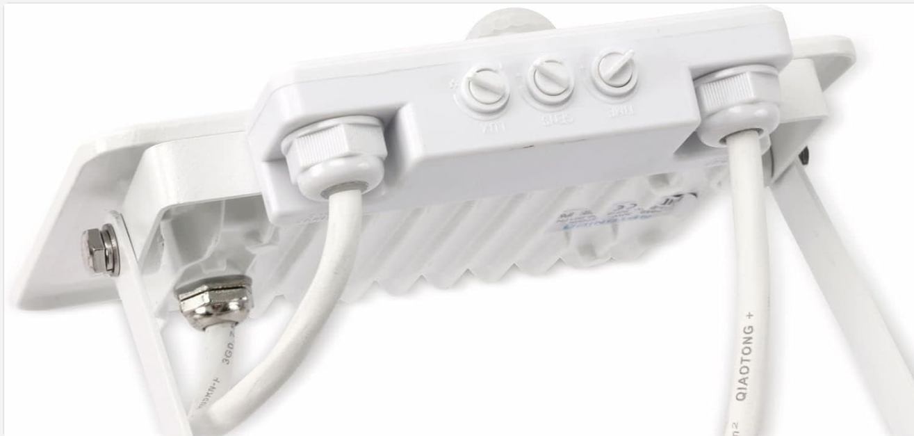
Image: Detailed view of the motion sensor's adjustment knobs. From left to right, these are typically for TIME, SENS (Sensitivity), and LUX (Light Level).
