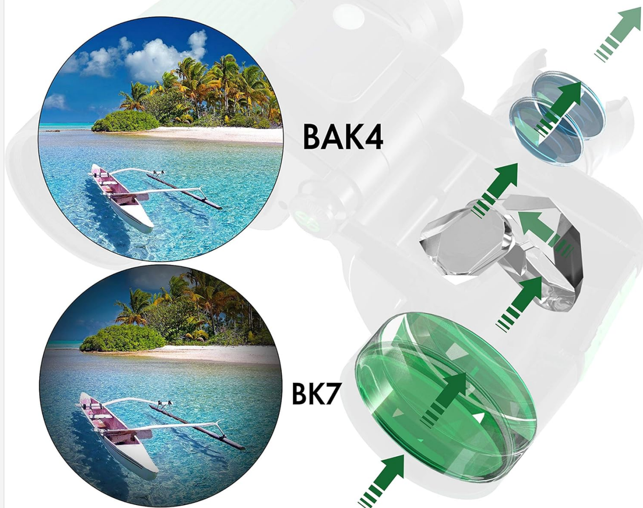
Image 2.1: Illustration of BAK4 prism providing better light transmission and clearer image compared to BK7.
