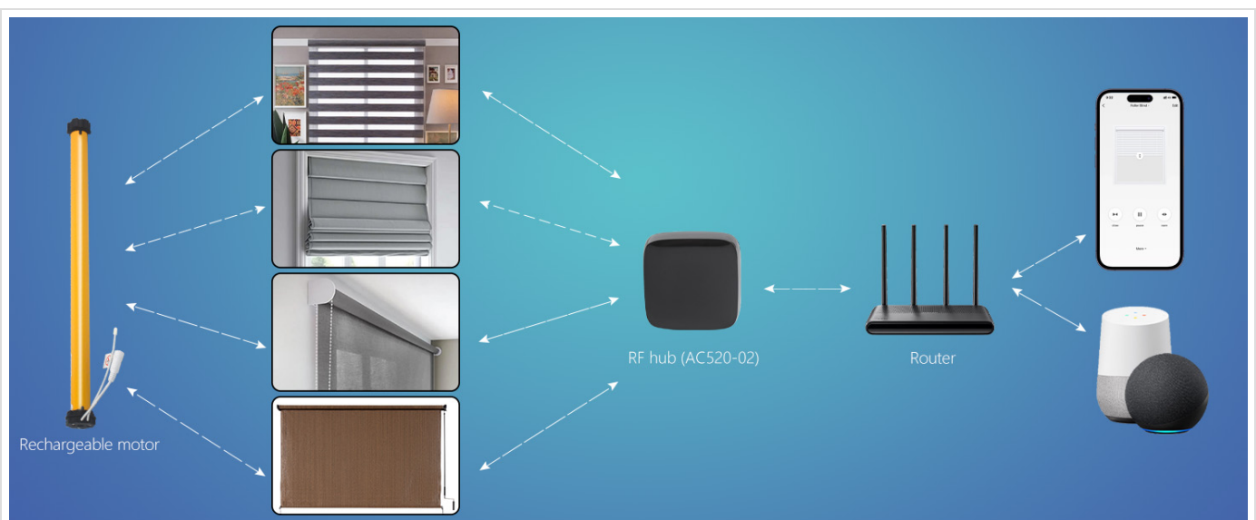
Figure 3.2: Voice Control Setup. This diagram shows how the motor can be controlled via voice commands using smart home devices like Amazon Alexa and Google Home, connected through a compatible RF hub.
