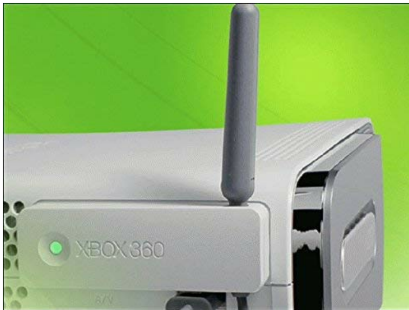
Figure 3.1: The Wireless Adapter connected to the rear USB port of an Xbox 360 console, showing the adapter's front with a green indicator light.
