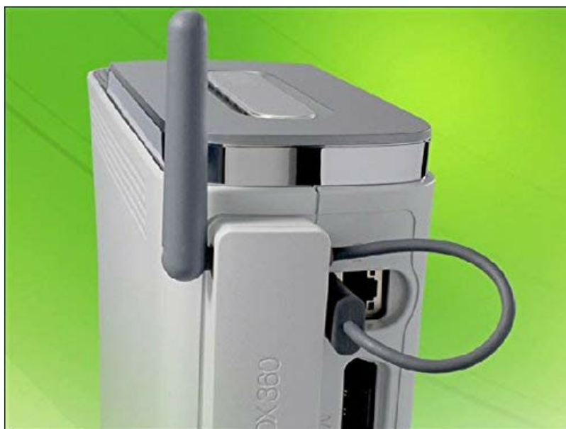
Figure 3.2: The Wireless Adapter connected to the Xbox 360, illustrating the cable routing and the antenna adjusted upwards.
