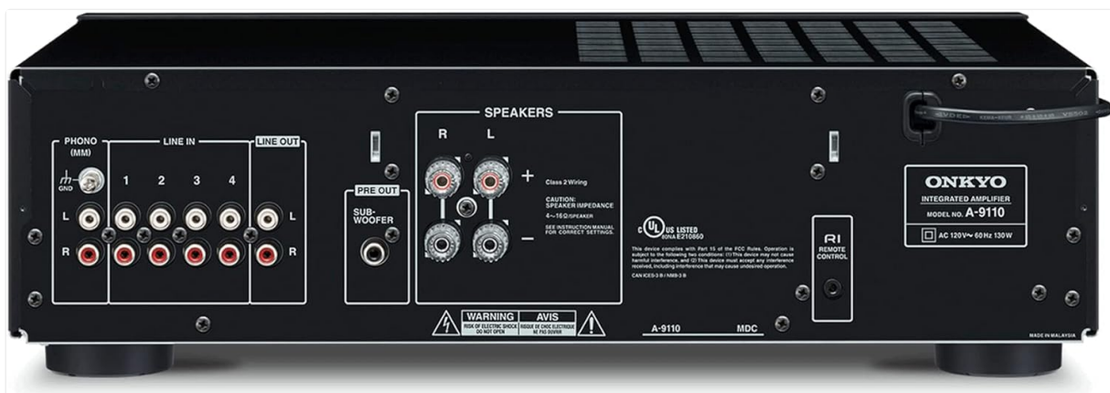
Image: Rear view of the Onkyo A-9110 amplifier, displaying the PHONO (MM) input, LINE IN 1-4, LINE OUT, PRE OUT, SUBWOOFER output, speaker terminals, and RI remote control jack.
