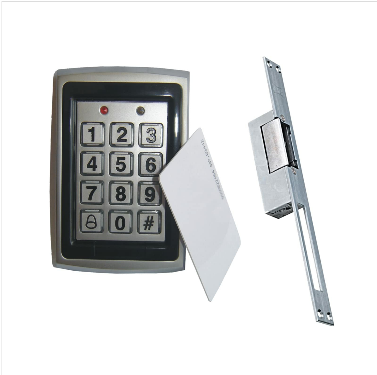
Figure 3.1: The Lorex LR-DPH2 Coded Card Door Access System, showing the keypad, card reader, and included electric lock strike and proximity cards. This image illustrates the main components of the access control kit.
