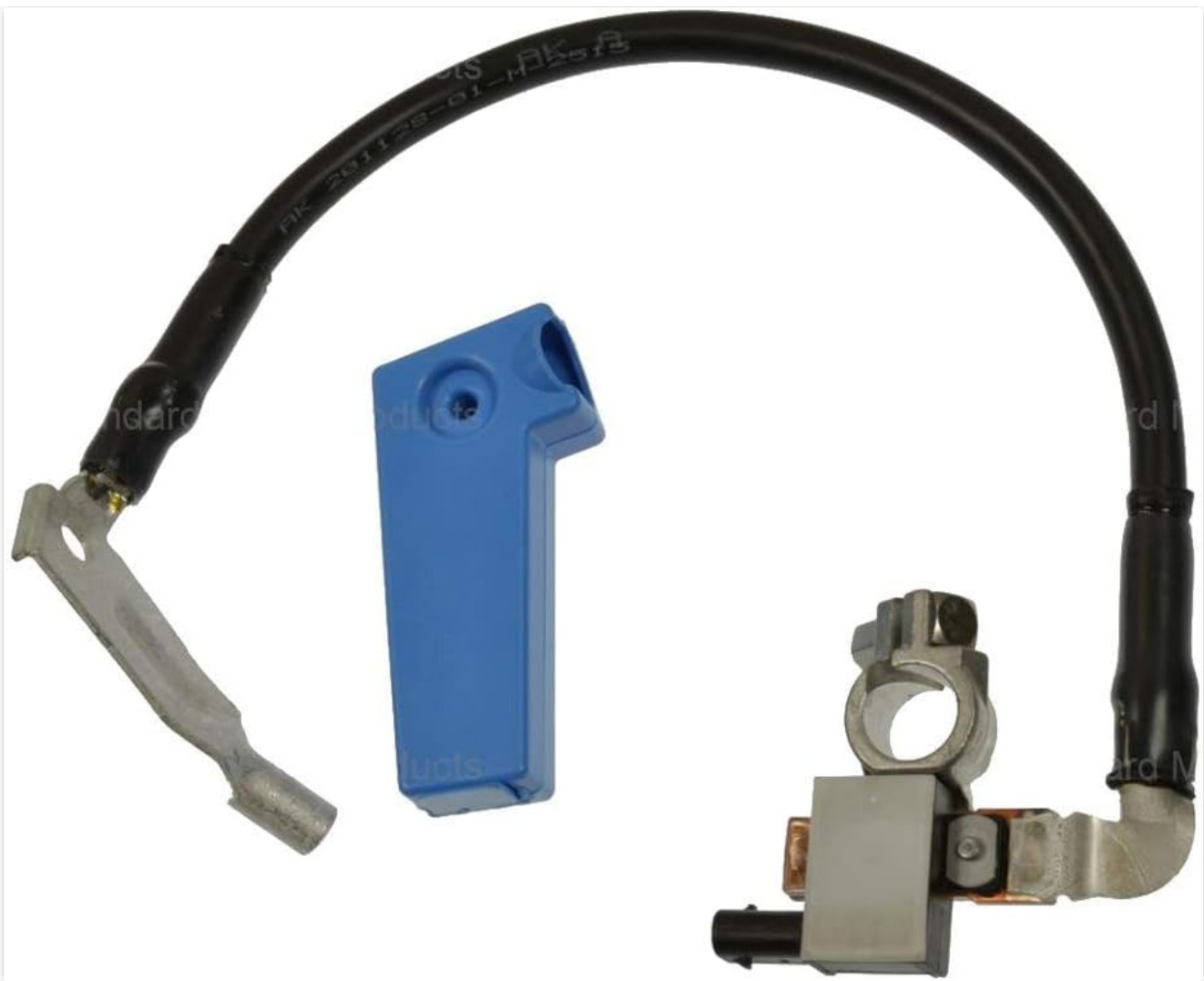
Figure 1: Full view of the Standard Motor Products BSC85 Battery Current/Volt Sensor, showing the main sensor unit, cable, and terminal connectors.
