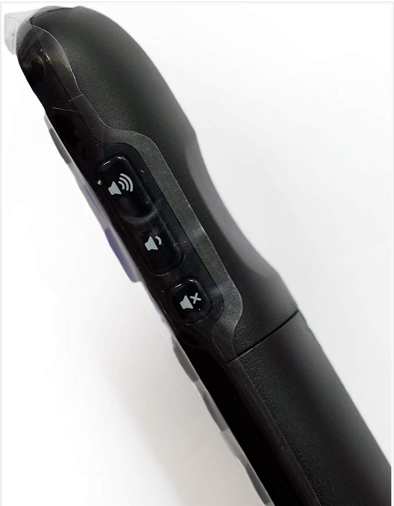
Image 4.1: Side view of the remote control, illustrating the placement of the volume up, volume down, and mute buttons.
