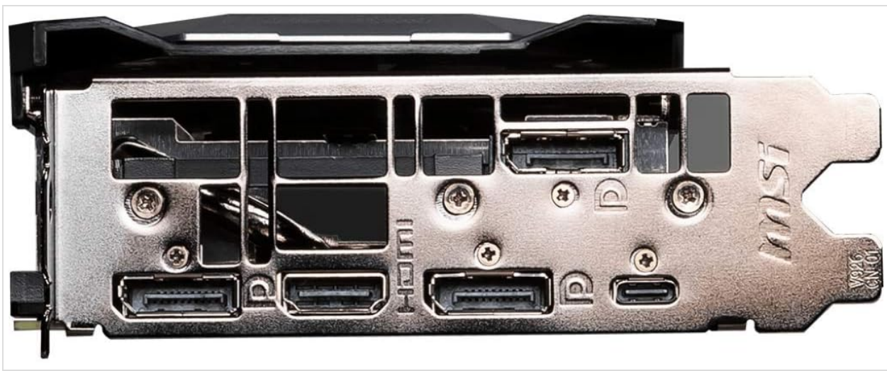
Figure 3.5: A close-up of the rear input/output panel, featuring multiple DisplayPort, HDMI, and USB Type-C connectors for display output.
