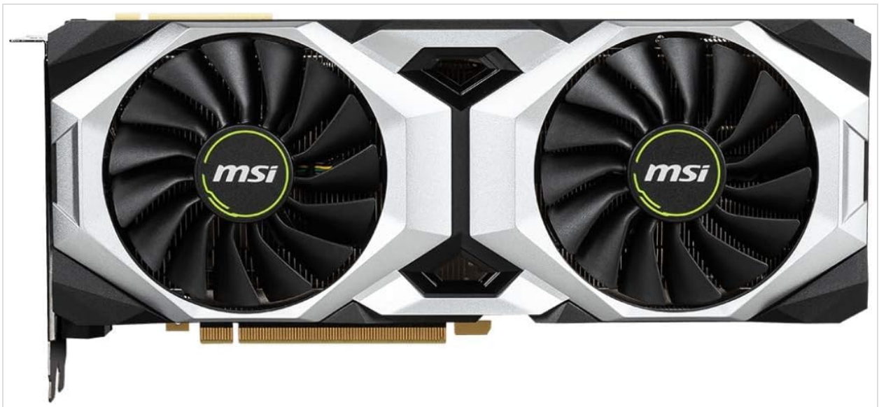
Figure 3.2: A direct front view of the graphics card, showcasing its dual-fan cooling system with MSI branding on the fan hubs and a silver and black shroud design.
