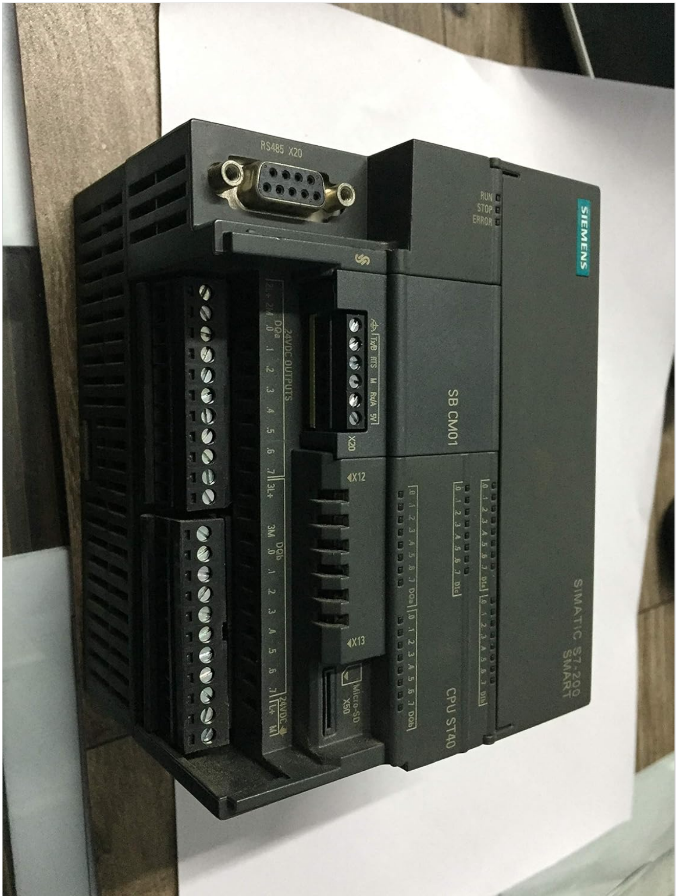
Figure 3: Top view of the Siemens ST40 S7-200 Smart PLC, illustrating the various input and output terminals, including the RS485 X20 port.
