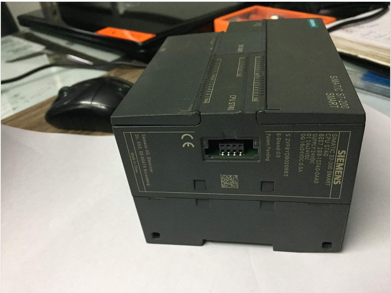
Figure 2: Side view of the Siemens ST40 S7-200 Smart PLC, highlighting the product label with model number and power specifications.
