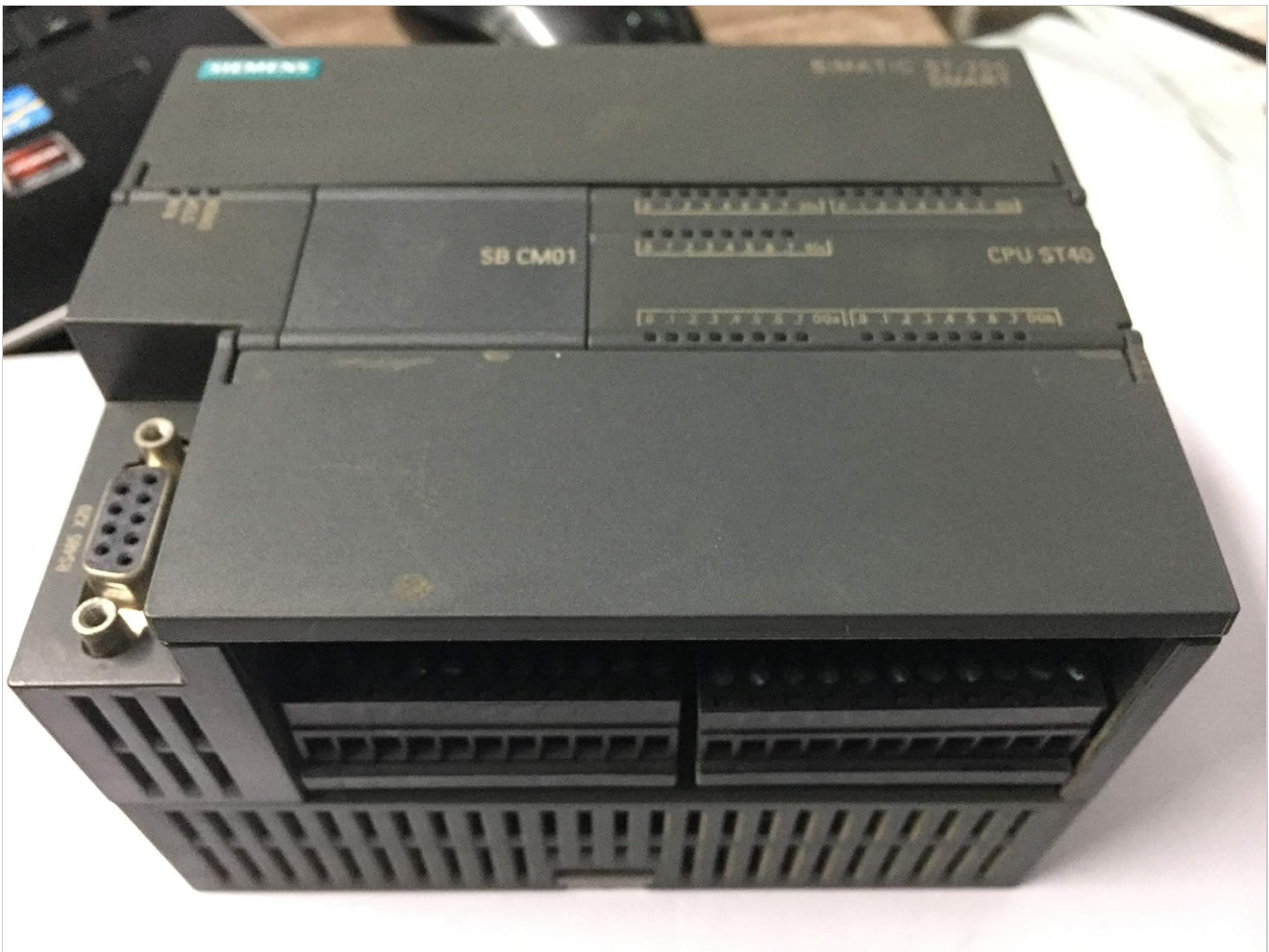
Figure 1: Front view of the Siemens ST40 S7-200 Smart PLC, showing the main unit with various ports and indicators.
