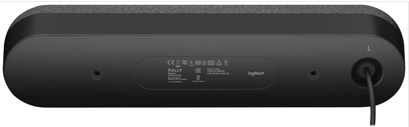
Rear view of the Rally Speaker, showing the power input and Mini XLR connection port.
