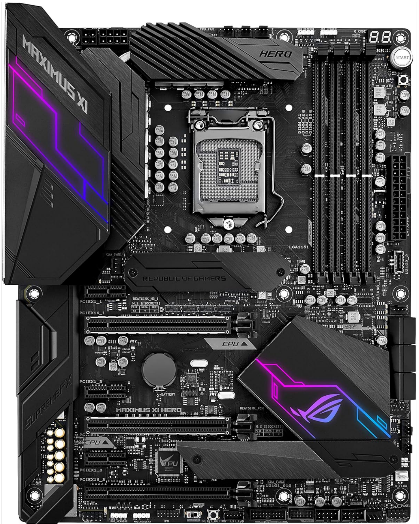
Figure 2.1: Close-up view of the LGA 1151 CPU socket on the motherboard, ready for processor installation.
