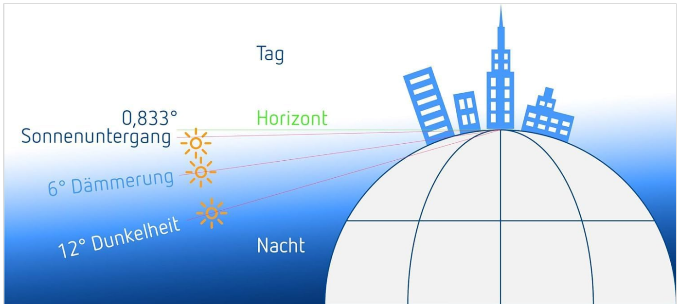
Figure 5.1: Diagram illustrating the astronomical function, showing how the timer calculates sunrise, sunset, and twilight periods (6° Dämmerung = 6° Twilight, 12° Dunkelheit = 12° Darkness) for precise light control.
