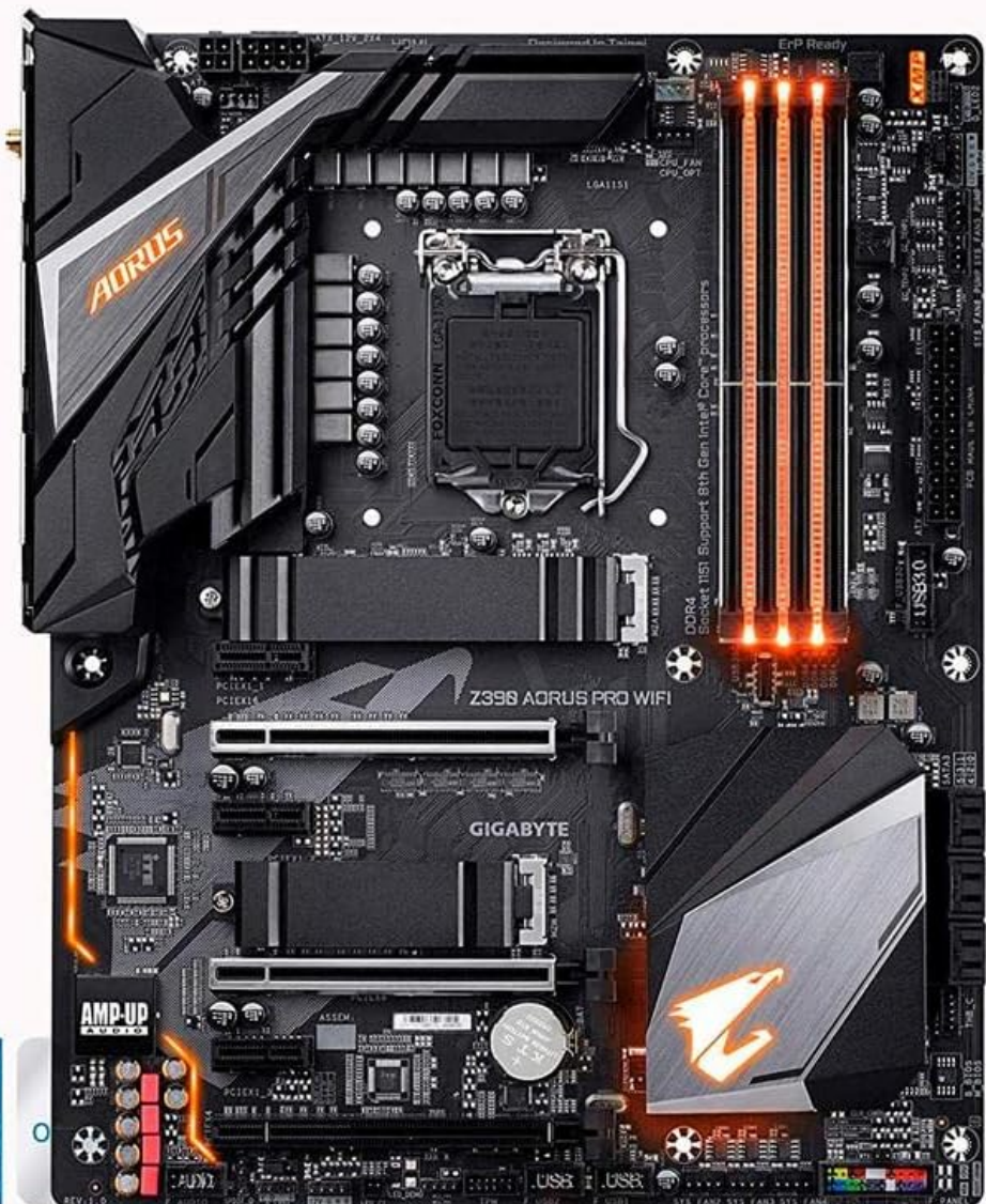
Image Description: A top-down view of the GIGABYTE Z390 AORUS PRO Wi-Fi Motherboard, illustrating the placement of the CPU socket, four DDR4 RAM slots, two M.2 slots with thermal guards, PCIe slots, and various headers for power and peripherals.
