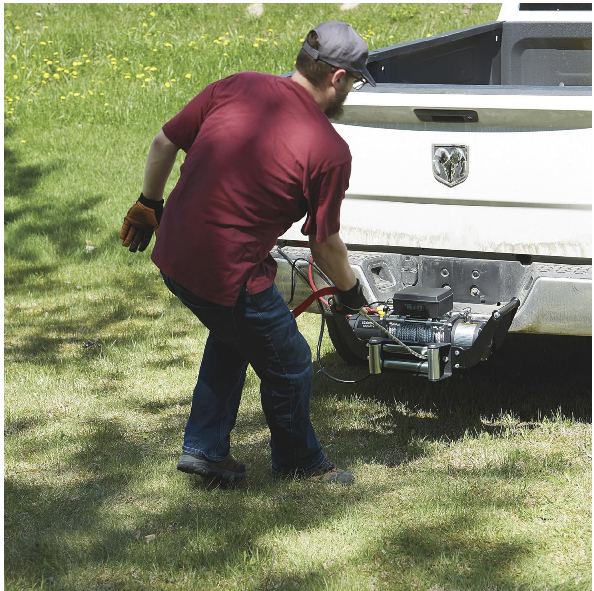
Image 4.3: A person preparing for a winching operation, standing near the Ironton winch mounted on a truck, demonstrating the typical setup before use.
