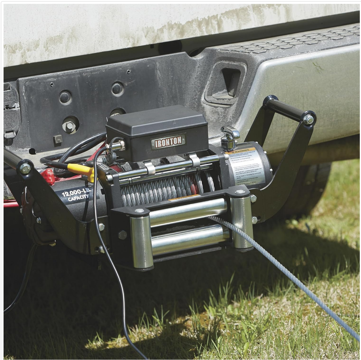
Image 3.1: The Ironton winch securely mounted on the rear of a truck, demonstrating proper installation with the wire rope guided through the roller fairlead.
