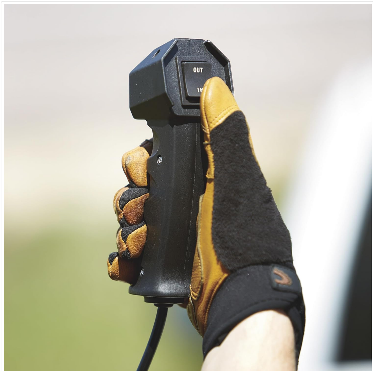
Image 4.1: A gloved hand pressing the 'OUT' button on the wired remote control, indicating the extension of the winch rope.
