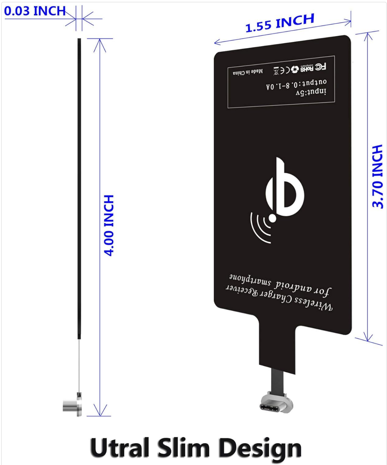
Figure 9: Ultra-Slim Design and Dimensions. This image provides the precise dimensions of the ultra-slim wireless charging receiver:
