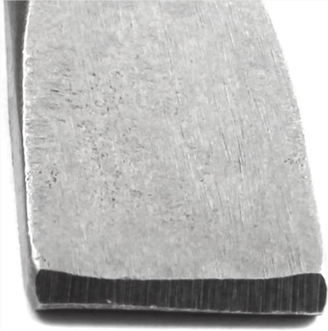
Figure 2: Close-up view of the 20mm wide flat chisel tip, designed for effective material removal.
