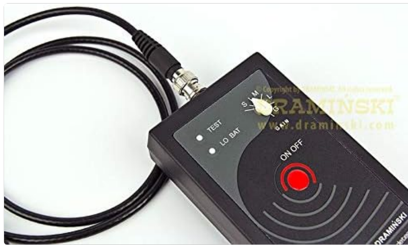
Figure 3.1: Detailed view of the detector's control panel, highlighting the gain adjustment and power controls.
