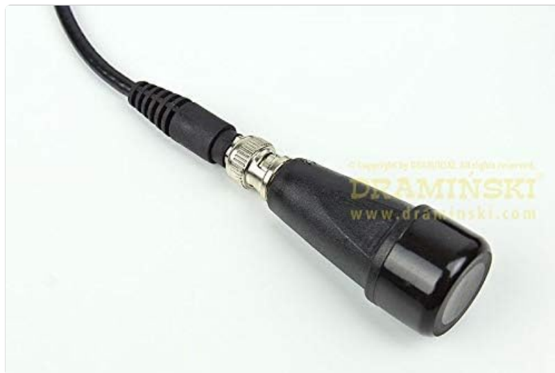
Figure 3.2: The ultrasonic probe, which is applied to the animal's skin for detection.
