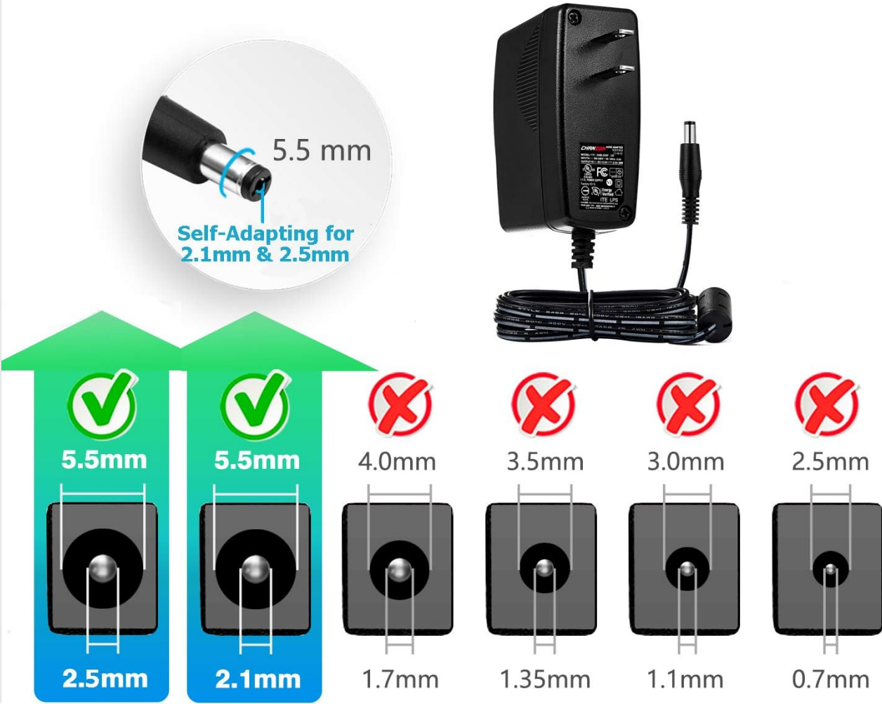
Image: Detailed view of the power supply, including its physical dimensions and the specifications of the DC barrel connector (5.5mm outer, 2.1mm/2.5mm inner diameter, center positive).
