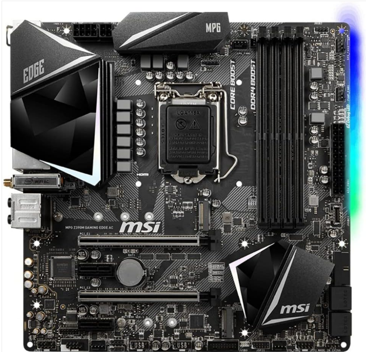
Figure 2: Top-down view highlighting the LGA 1151 socket, DDR4 slots, and M.2 slots.
