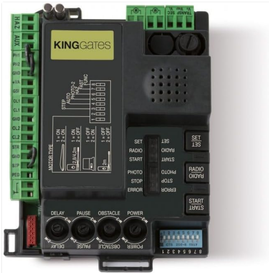
Figure 3.1: Front view of the King Gates STARG8 24 electronic board. This image displays the various terminals for connections, DIP switches for configuration, and control buttons for programming and manual operation. Key areas include motor type selection, photocell settings, and functional DIP switches.
