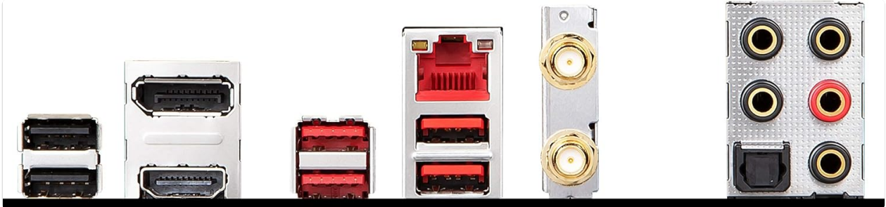
Figure 5: Rear I/O panel of the motherboard, showing USB ports, HDMI, DisplayPort, Ethernet, Wi-Fi antenna connectors, and audio jacks.
