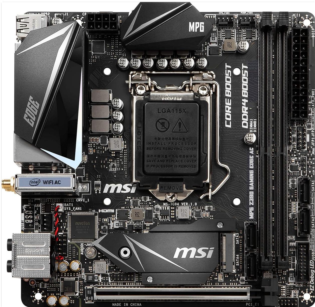
Figure 4: Detailed view of the LGA 1151 CPU socket, showing the protective cover and retention mechanism.
