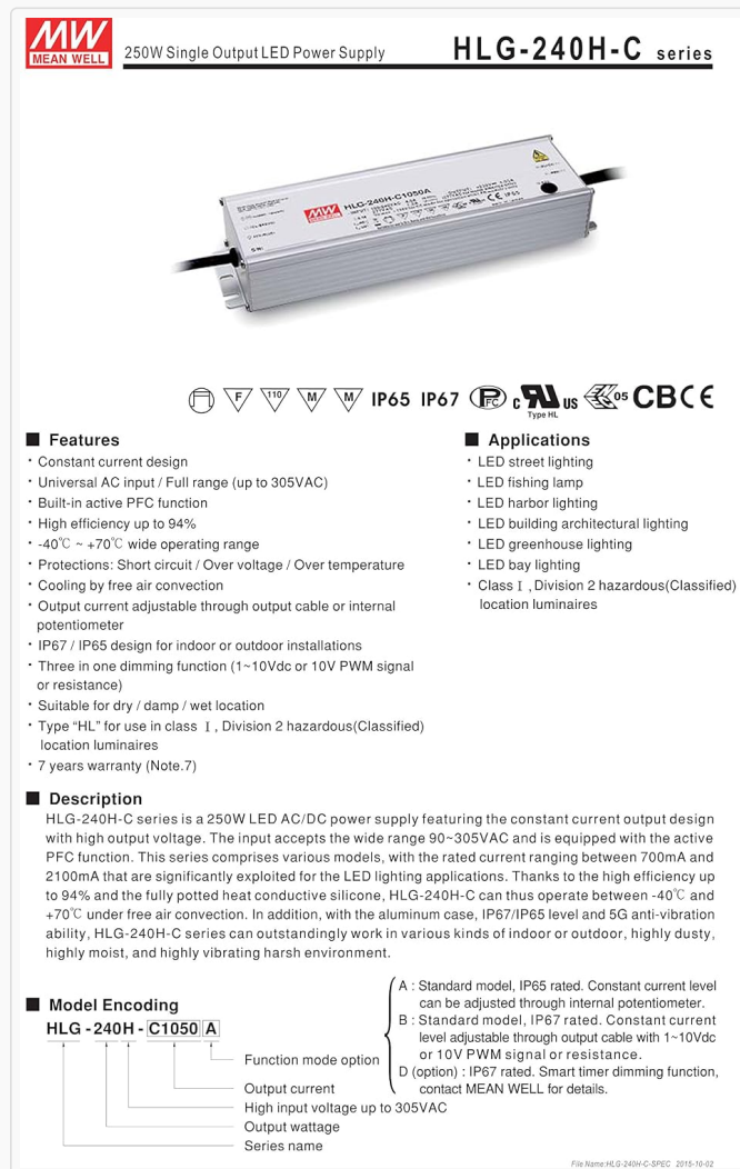
Figure 2.1: Diagram illustrating the key features and typical applications of the HLG-240H-C series LED power supply.
