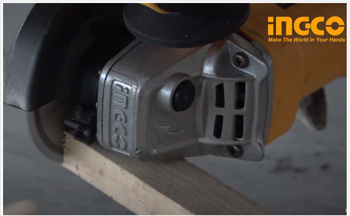
Figure 4.1: Demonstrating the angle grinder in use for cutting wood. Observe the proper grip and direction of sparks, indicating safe operation.
