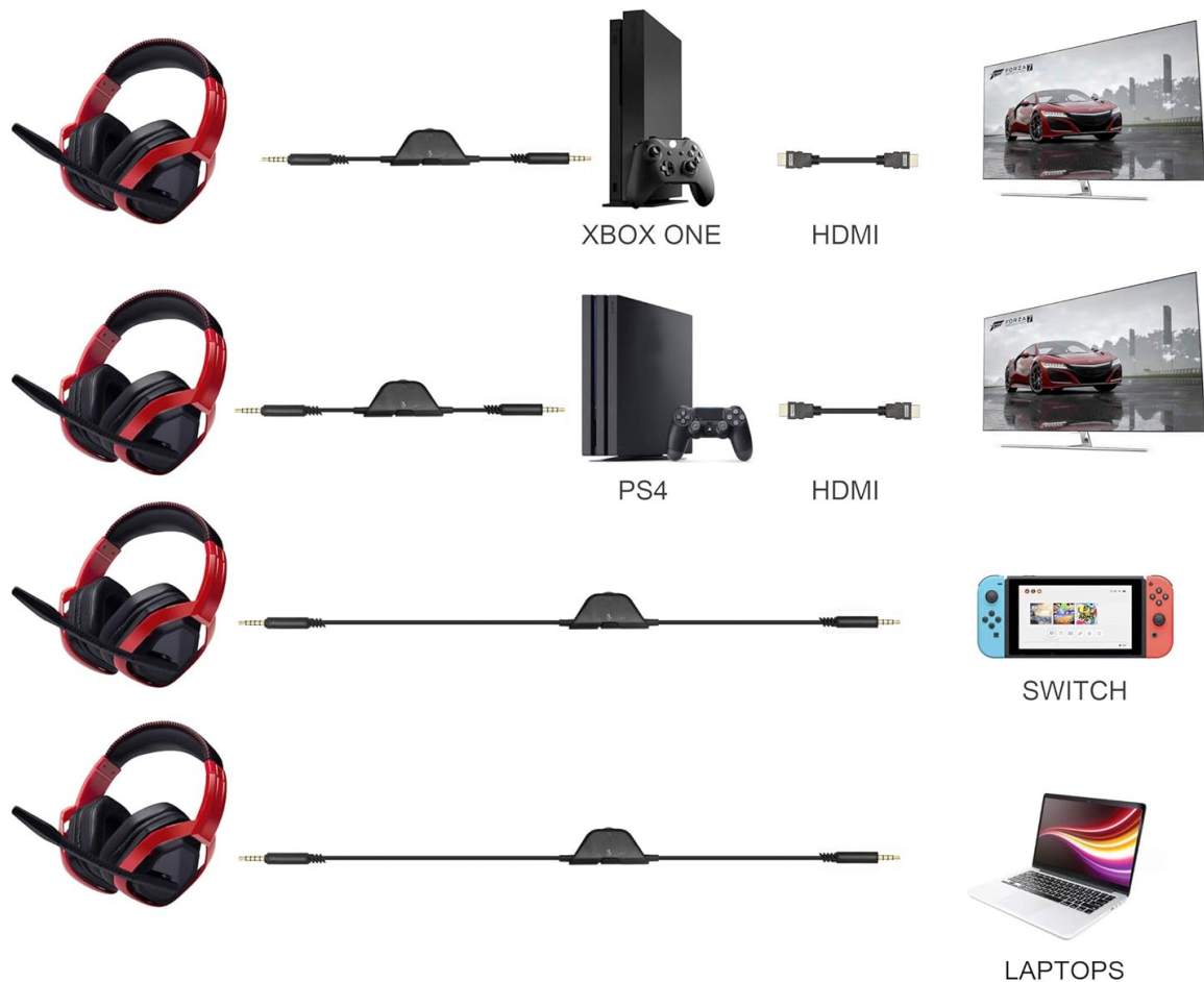
Image: Diagram illustrating how to connect the headset to Xbox One, PS4, Nintendo Switch, and Laptops.
