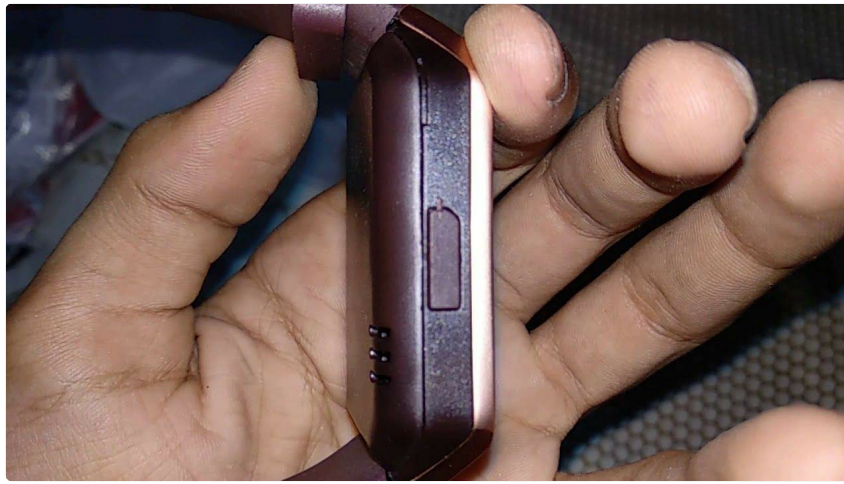
Figure 4.1: Illustration of the SIM and TF card installation area on the back of the watch.
