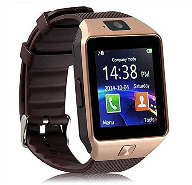
Figure 3.1: Front view of the ANITECH DZ09 Smart Watch, showing the display, camera, and side button.
