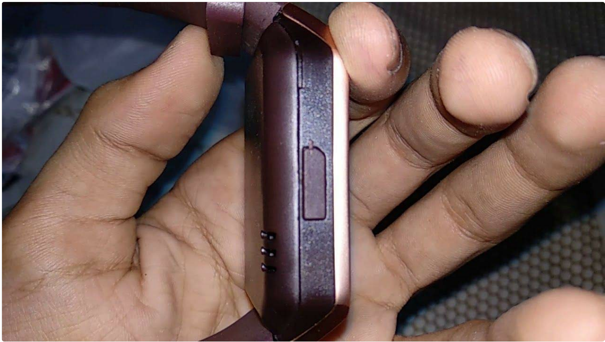
Figure 3.4: Detailed view of the smart watch's back panel, revealing the SIM card and TF card slots for expansion.
