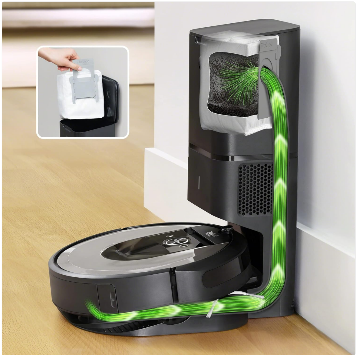
Image: A hand demonstrates inserting a new iRobot dirt disposal bag into the Clean Base unit. The diagram shows the path of dirt from the Roomba into the bag.
