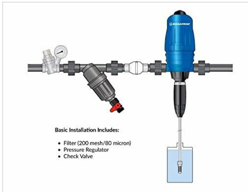
Figure 2: Basic installation diagram for the Dosatron D14MZ2. This diagram illustrates the doser connected to a water line, with a filter, pressure regulator, and check valve installed upstream for system protection and performance.
