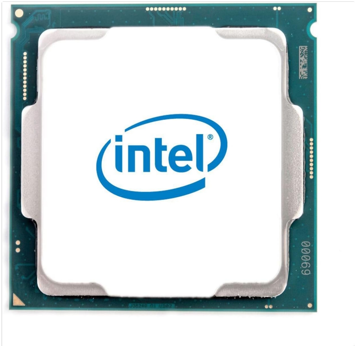
Image 2.1: Top view of the Intel Core i7-9700K processor, showing the integrated heat spreader.
