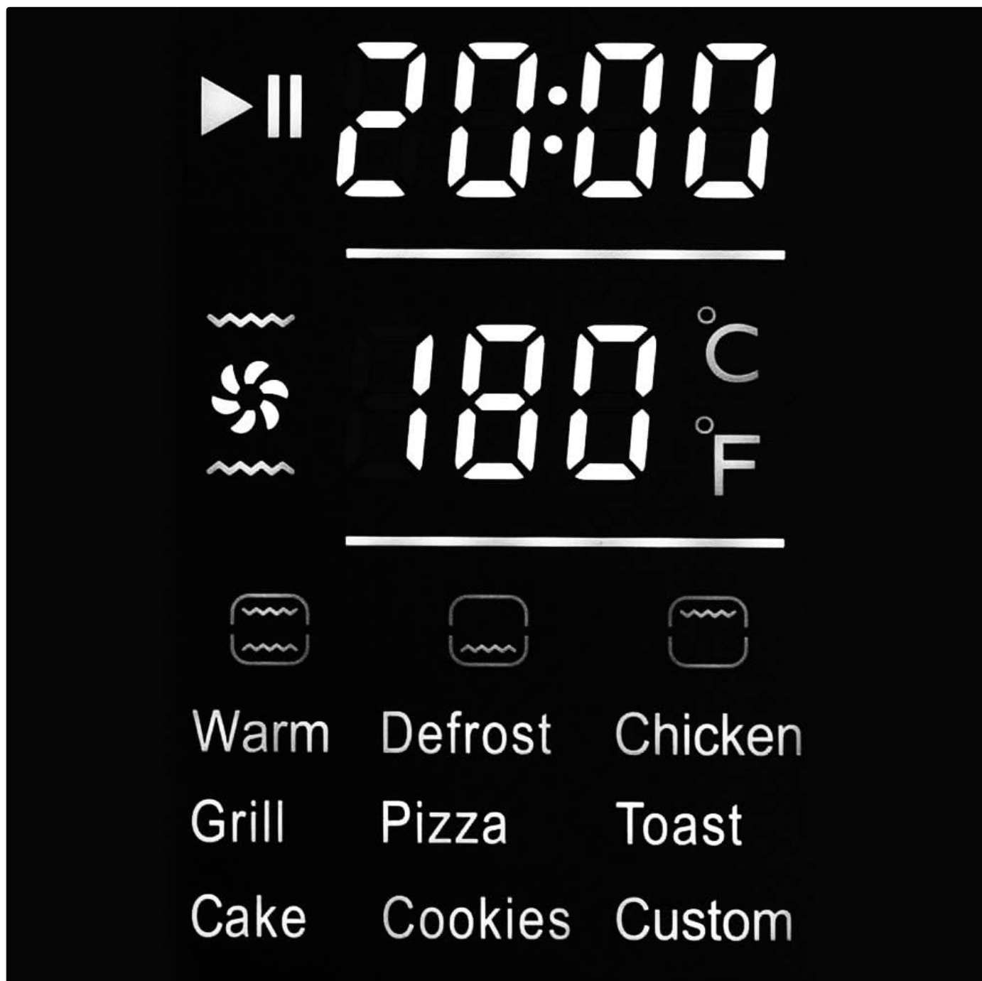
Figure 4.1: Detailed view of the backlit touch display, showing program icons, temperature, and time settings.
