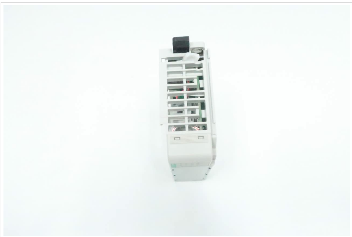
Figure 3.2: Side view of the 1769-OB16 module, illustrating its compact design.
