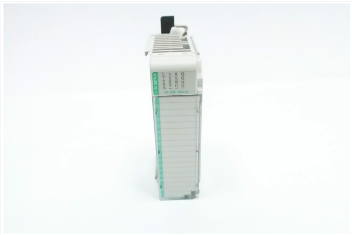
Figure 3.1: Front view of the 1769-OB16 module, showing the output terminals and status indicators.
