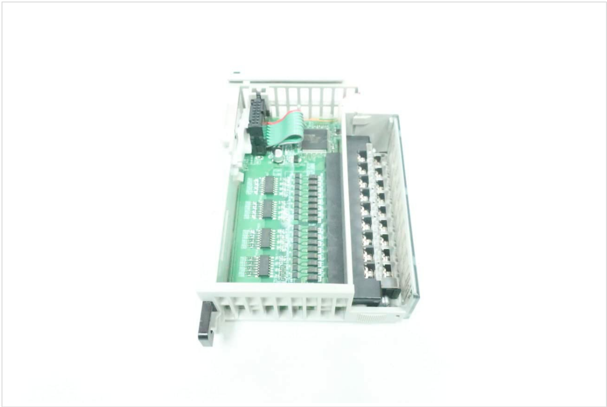
Figure 3.3: Internal view of the 1769-OB16 module, showing the circuit board and connectors.
