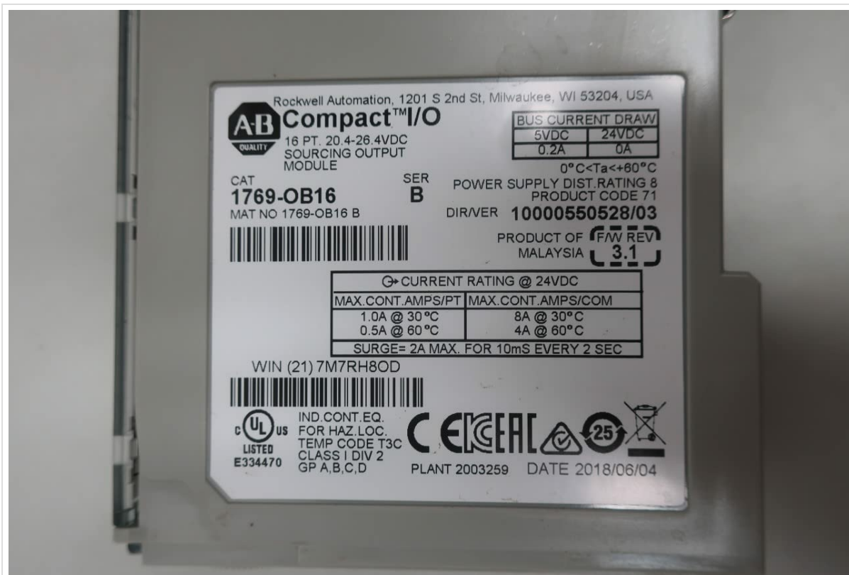
Figure 3.5: Product label for the 1769-OB16 module, detailing electrical ratings and certifications. Key information includes: CAT 1769-OB16, SER B, BUS CURRENT DRAW 5VDC 0.2A, 24VDC 0A, MAX CONT AMPS/PT 1.0A @ 30°C, 0.5A @ 60°C, MAX CONT AMPS/COM 8A @ 30°C, 4A @ 60°C, SURGE = 2A MAX. FOR 10ms EVERY 2 SEC. The code 217M7RH8OD is also visible. More information on Rockwell Automation website.
