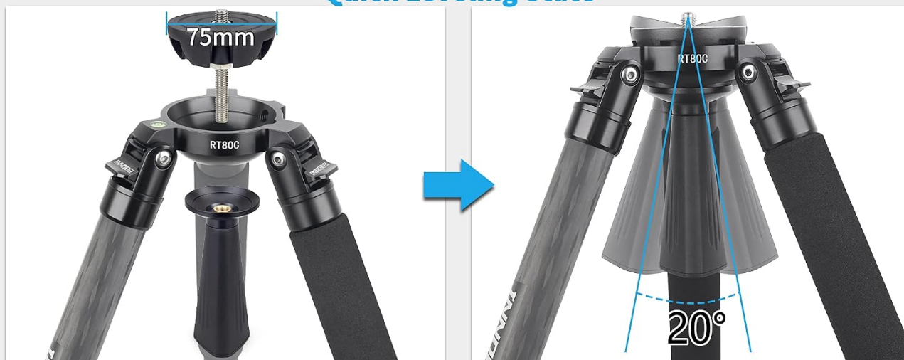
Figure 4: Mounting Plate Options. This image demonstrates how to switch between the normal flat plate mounting state and the quick leveling state using the 75mm bowl adapter. The top plate is 80mm in diameter, and the bowl adapter is 75mm.
