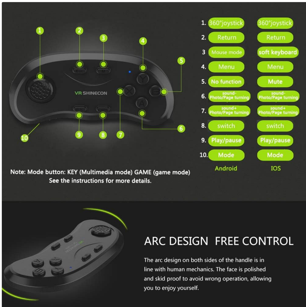
Image: A detailed diagram of the VR SHINECON remote controller, labeling its various buttons and their corresponding functions, including joystick, return, mouse mode, menu, mute, volume/page controls, switch, play/pause, and mode selection for Android/iOS.
