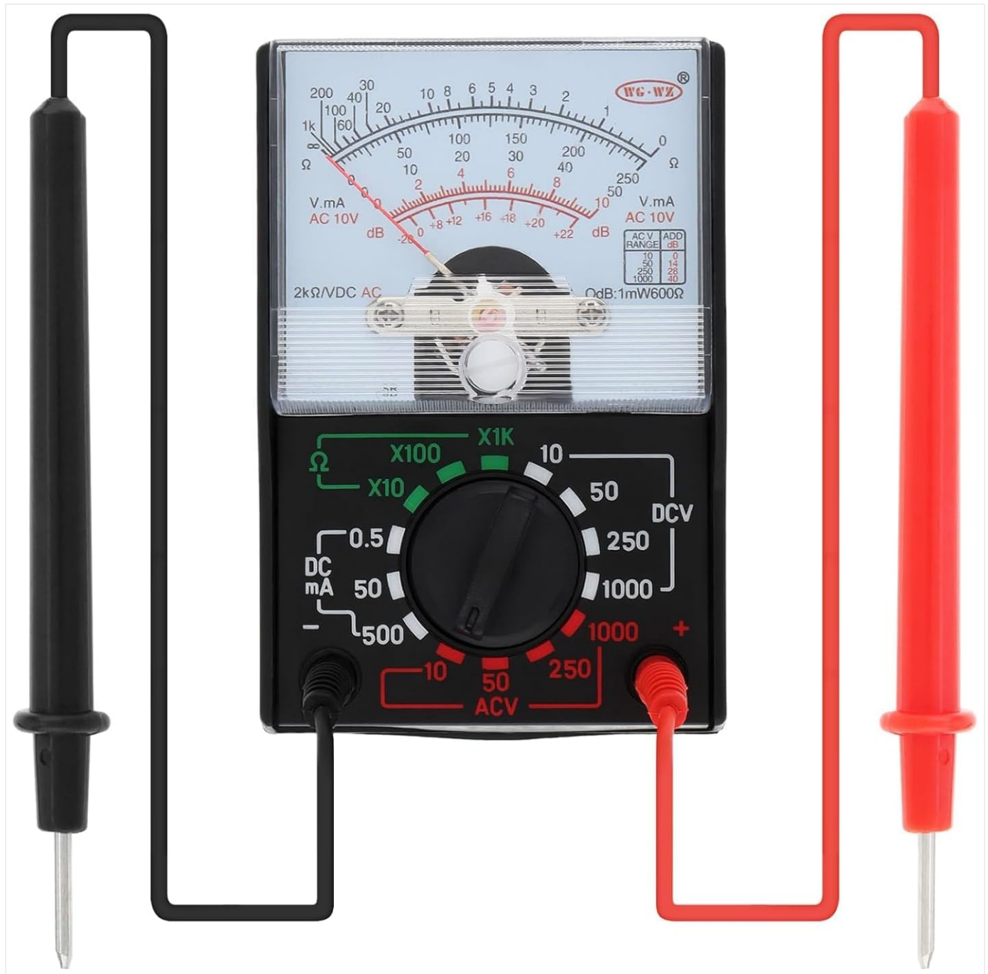
Figure 6: The multimeter with the red test lead connected to the positive input and the black test lead connected to the common ground.
