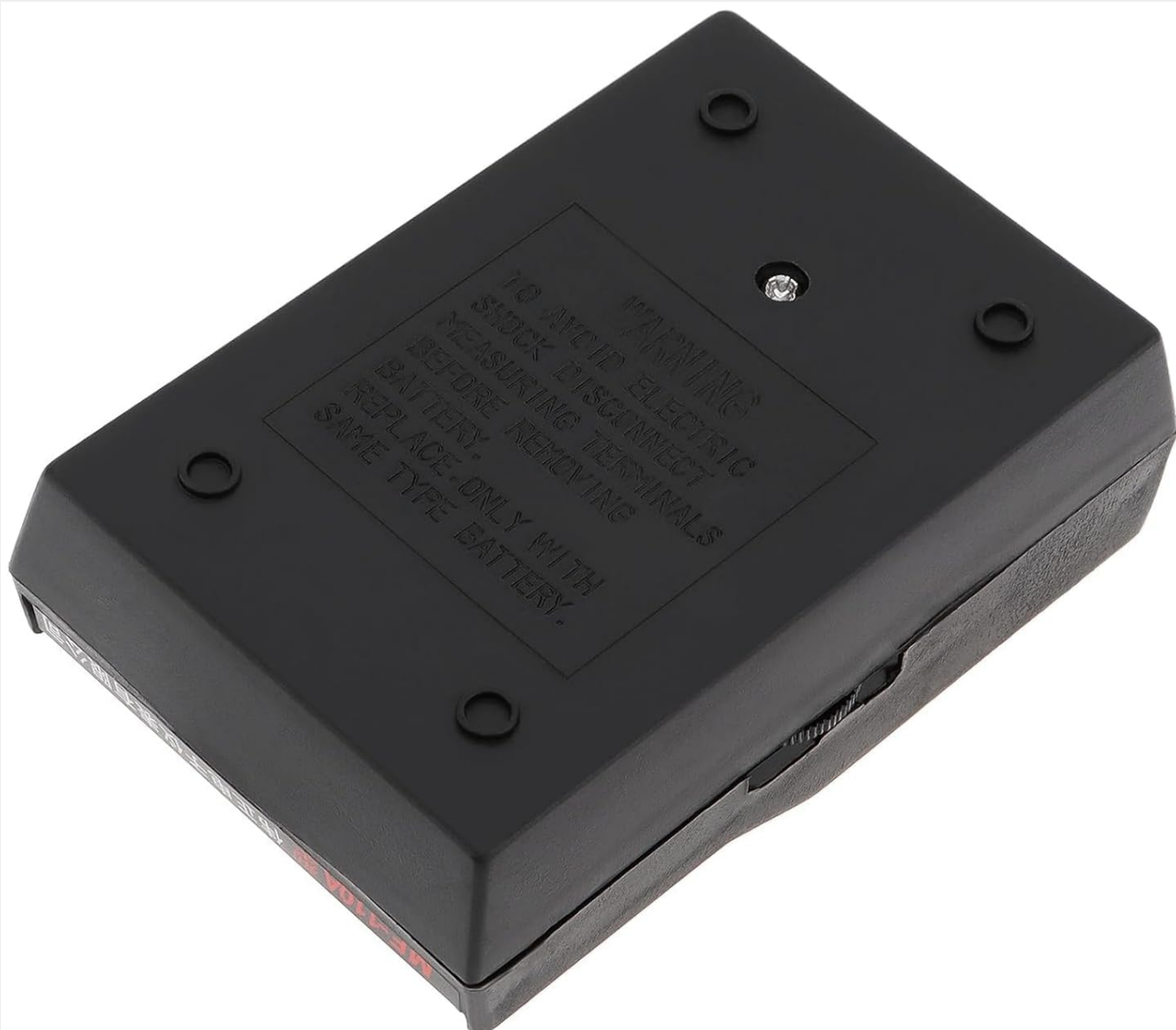
Figure 1: Back of the multimeter with a warning label. The label states: "WARNING TO AVOID ELECTRIC SHOCK DISCONNECT MEASURING TERMINALS BEFORE REMOVING BATTERY. REPLACE ONLY WITH SAME TYPE BATTERY."
