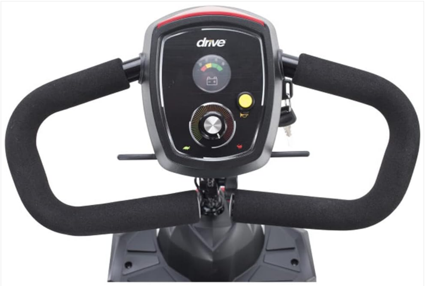
Figure 3: Detailed view of the delta tiller, control panel with battery indicator, speed adjustment dial, and horn button.
