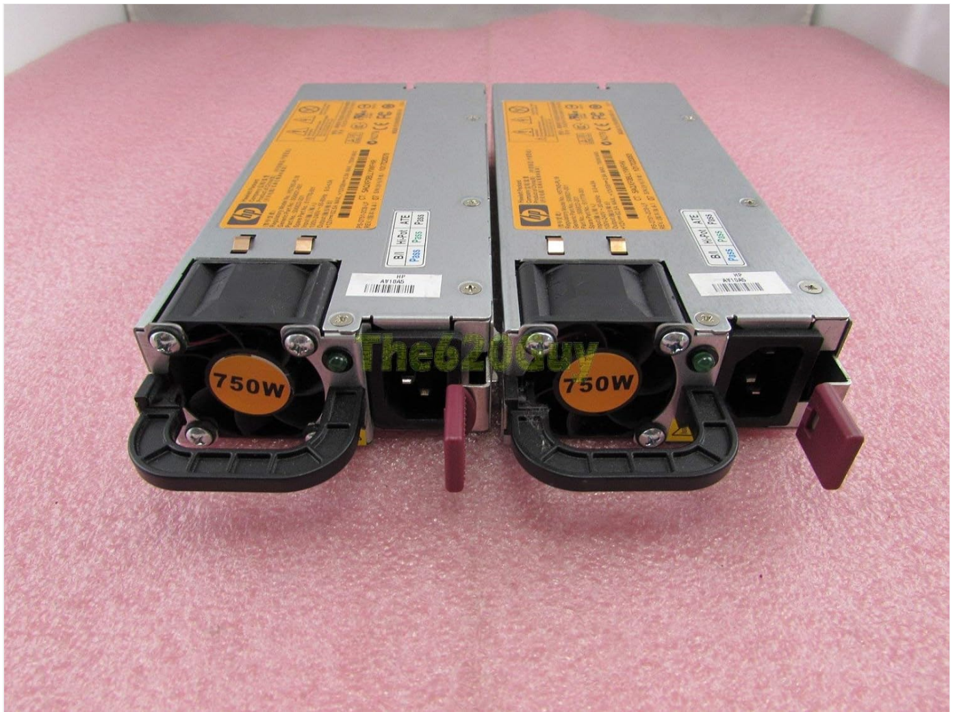
Image 2.3: Front view of two HP 750W PSUs, illustrating the cooling fans labeled "750W" and the AC power input receptacles.
