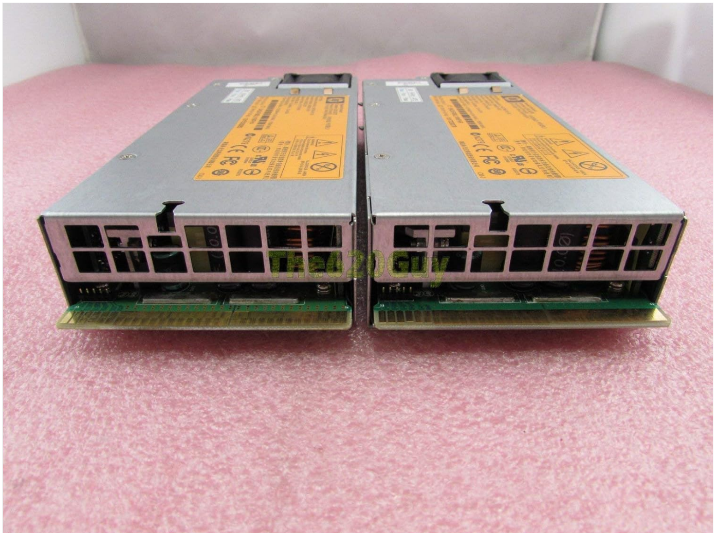
Image 2.4: Rear view of two HP 750W PSUs, displaying the gold-plated electrical connectors that interface with a server backplane or breakout board.
