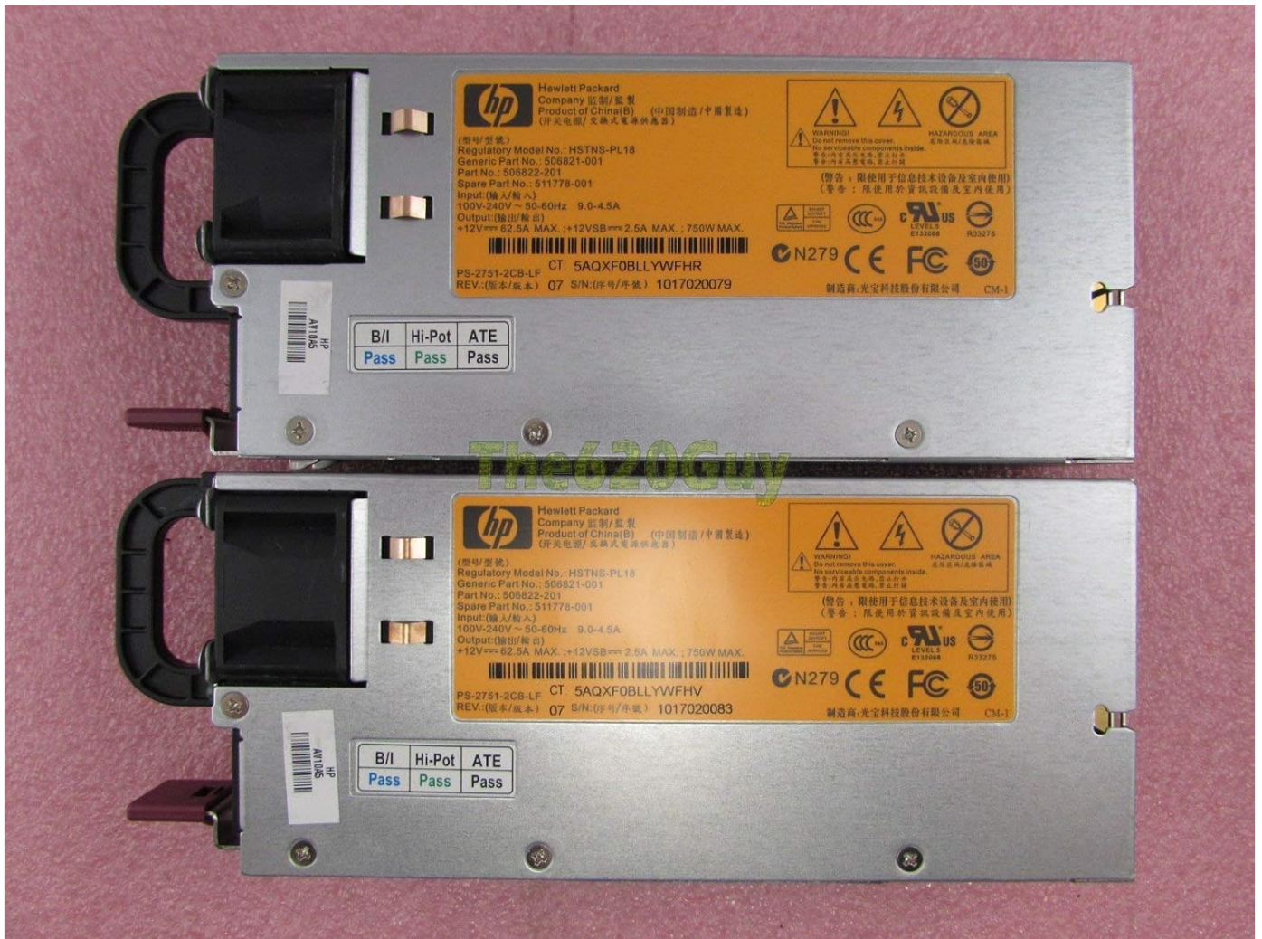
Image 2.1: Top view of two HP 750W PSUs, highlighting the regulatory model number HTSNS-PL18 and various part numbers including 506821-001, 506822-201, and 511778-001. The serial number 5AQXF0BLLYWFHR is visible on one unit.
