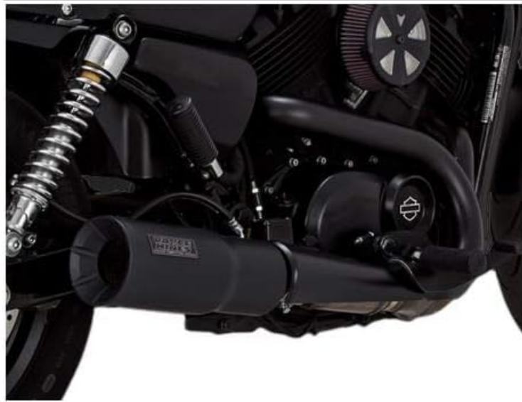
Figure 1: Vance & Hines 47943 Hi-Output Slip-On exhaust installed on a motorcycle. This image displays the Vance & Hines 47943 Hi-Output Slip-On exhaust system mounted on a motorcycle. The exhaust features a matte black finish with the Vance & Hines logo visible on the muffler body. The design is a short, aggressive style, complementing the motorcycle's overall aesthetic.
