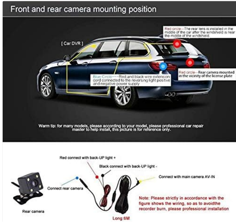
Image 3.2: Diagram illustrating recommended front and rear camera mounting positions and wiring connections.
