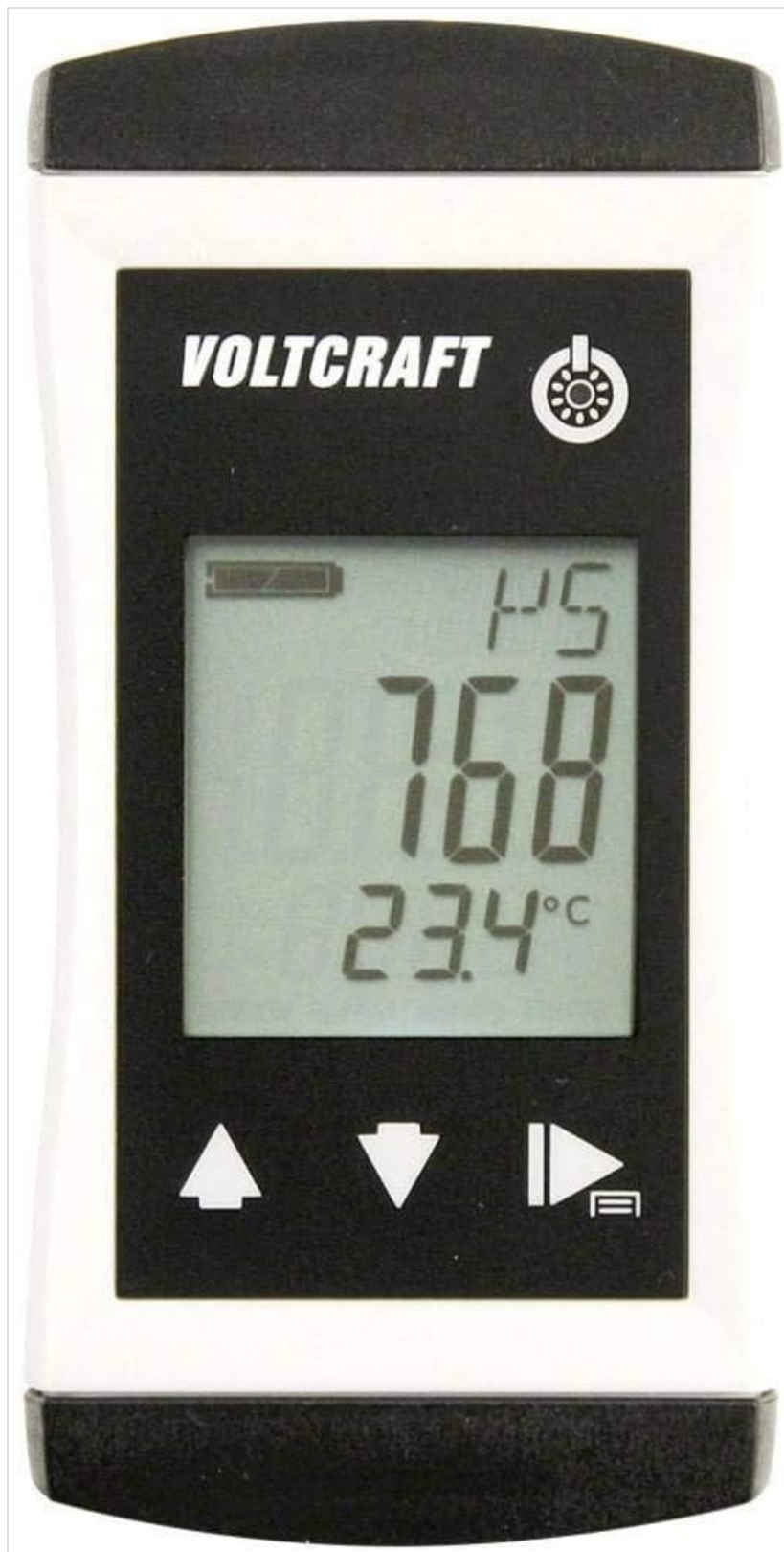
Figure 1: Front view of the LWT-100 Conductivity Meter. The device features a clear digital display showing conductivity and temperature readings, along with intuitive control buttons for navigation.
