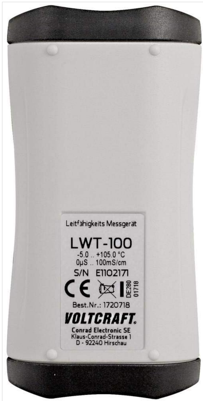
Figure 2: Back view of the LWT-100 Conductivity Meter. The rear label provides essential product information, including the model name, measurement range, and serial number.
