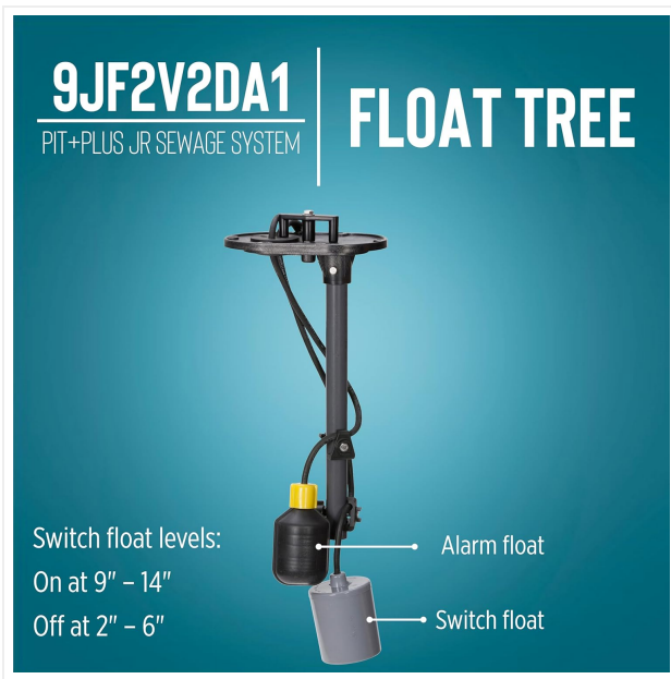
Figure 3.5: Float Tree and Switch Levels.
