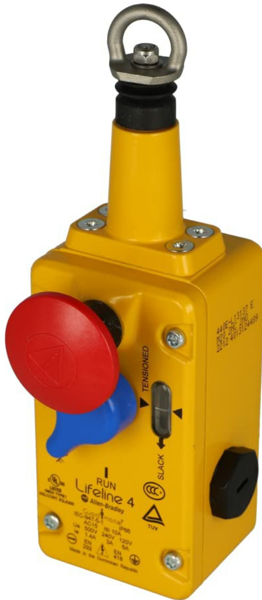
Figure 1: Guardmaster Lifeline 4 Cable Pull Switch. This image shows the yellow industrial safety switch with a red emergency stop button, a blue reset lever, and a cable tension indicator. The top features a metal eyelet for cable attachment, and the side displays product labeling.
