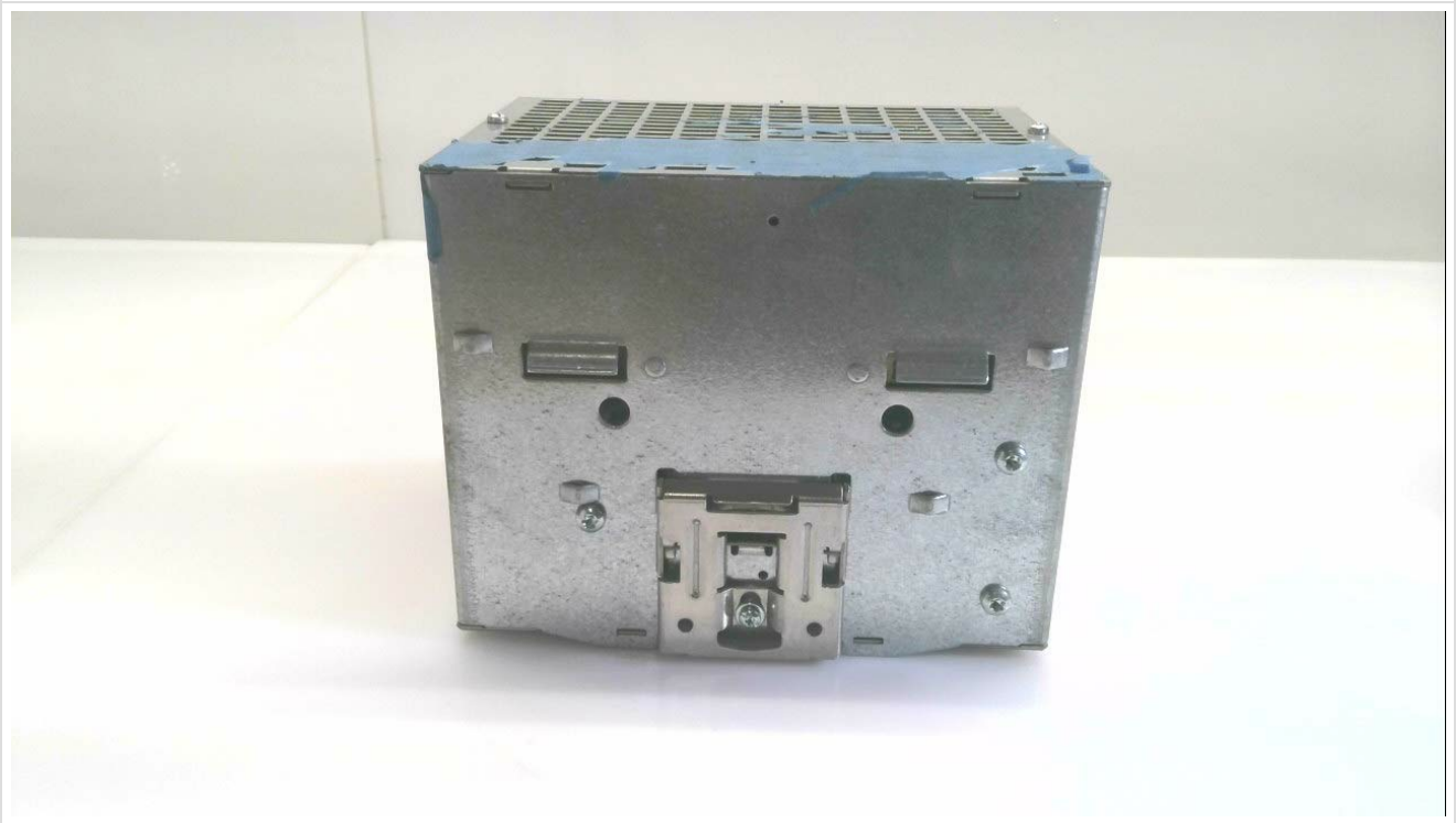
Figure 1: Rear view of the power supply, illustrating the plug-in mounting mechanism.
