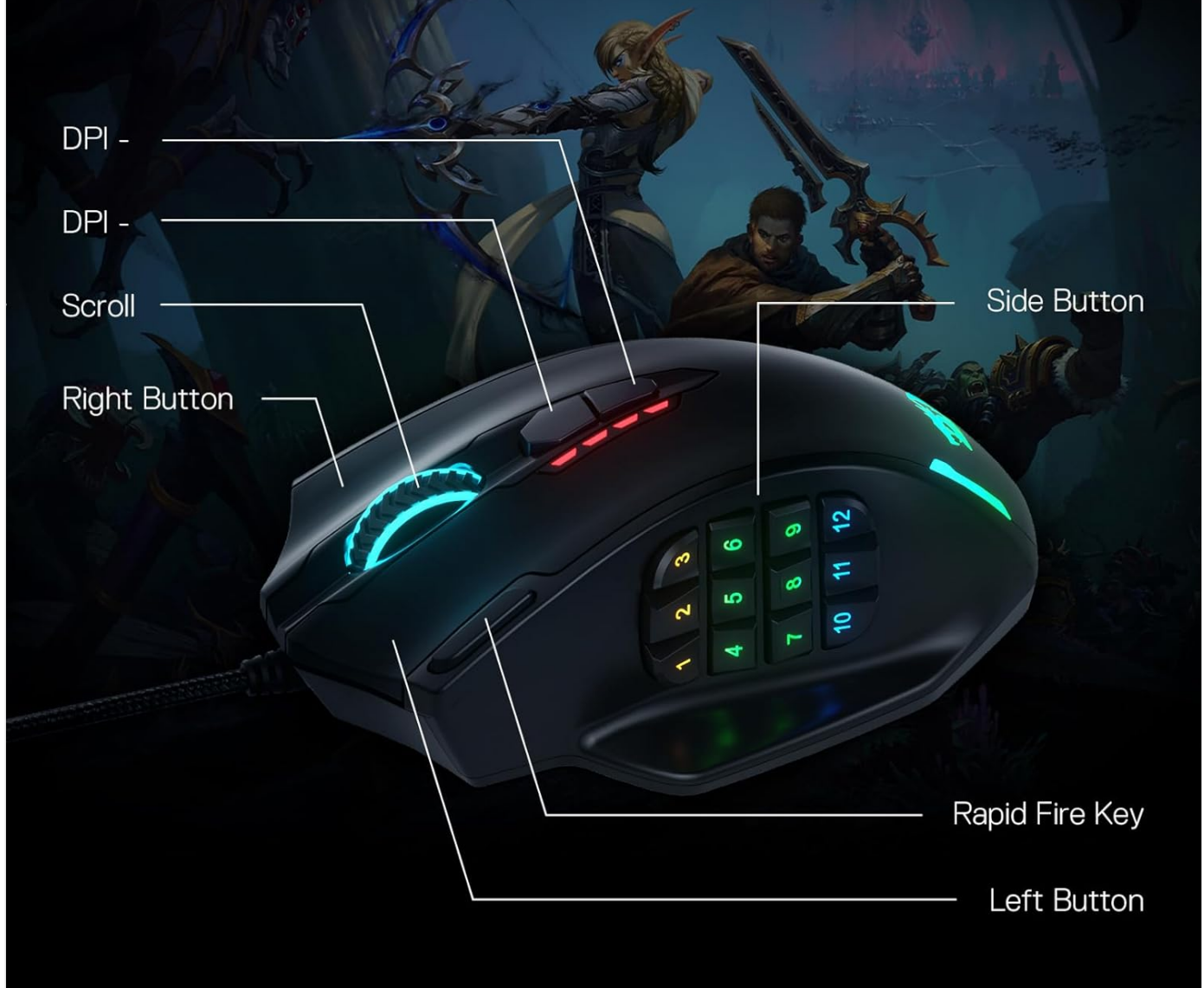
Figure 5: Detailed diagram of the 18 programmable buttons.
