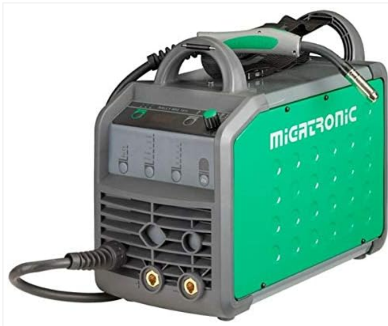
Front view of the MIGATRONIC Rallymig 161i multi-process welder, showing the control panel, output terminals, and integrated handle. The machine features a grey and green casing with the MIGATRONIC logo prominently displayed.
