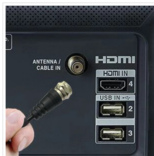
Image: A hand connecting the F-type coaxial cable to the 'Antenna/Cable In' port on the back of a television.
