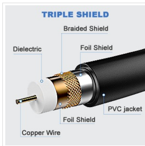
Image: Cross-section diagram illustrating the triple-shielded construction of the coaxial cable, including copper wire, dielectric, foil shield, braided shield, and PVC jacket.
